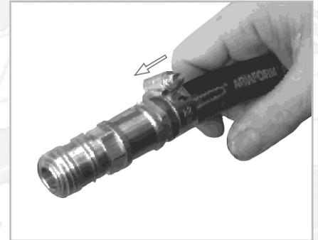
3. Move the clamp over the tube and the pillar of the coupling.
