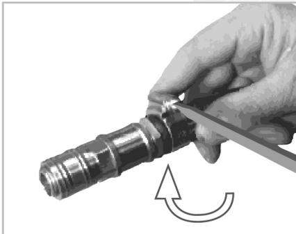
4. Turn the screw of the clamp to the right and fixate the clamp.
