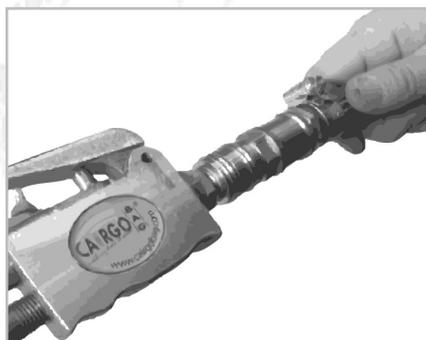
3. "Click", now the air tool is connected to the air tube.
