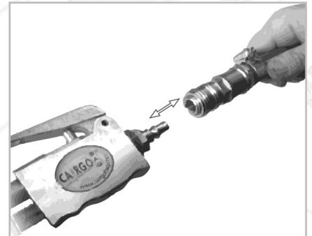
2. Put the connector of the air tool into the quick coupling. Press them firmly together.
