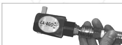
3. "Click", now the valve connector is connected to the air tool.
