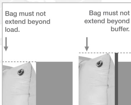
5. Buffer material should extend slightly beyond the load.
